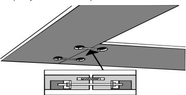
**Joins**Joins have to be made with jointing bolts and a strip. Use 2 bolts for a 650mm board.
