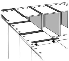
When installing on a cabinet with a full top, place 4-6mm thick sticks on top of the cabinets. Drill 2-3 holes in the top rear of the cabinets allowing the air to circulate.
