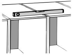
For the worktops to function perfectly it is essential that all kitchen units have been installed correctly with a spirit level so the upper surfaces are completely level.
