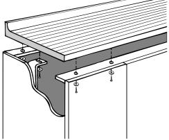
The worktops should be installed with a row of 3 screws each 300-500mm apart using supporting brackets in between where cabinets do not have a full top.
