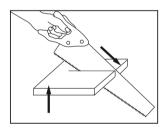
If using a hand saw, (10 to 12 teeth per 25mm) cut the worktop face up. Always start from the profiled front edge and keep the saw at a low angle.
