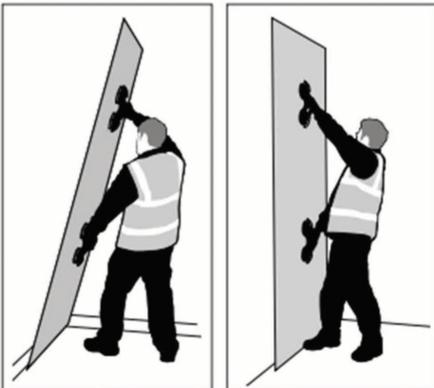
Ensure the bottom edge is correctly in place then push the panel back firm against the wall and apply pressure to all areas of the panel to make sure the TopSeal adhesive grabs to the wall.
