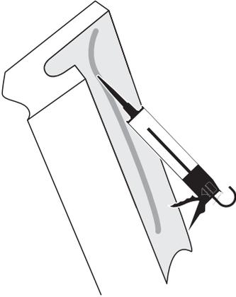
Once inserted, flatten the panel against the wall and smooth any excess adhesive across the joint to cover any missed areas.
