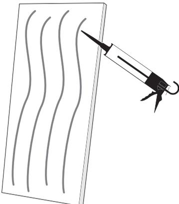
Before applying TopSeal, clean the edges or tongues and grooves to remove any dust that may interfere with the sealing process. Ensure that when joining two panels, the surface is flat to avoid any issues during the installation process.
